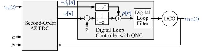
Fig. 1. High-level block diagram of a second-order  $\Delta\Sigma$  FDC-based digital fractional- $N$  PLL with quantization noise cancellation (QNC).
