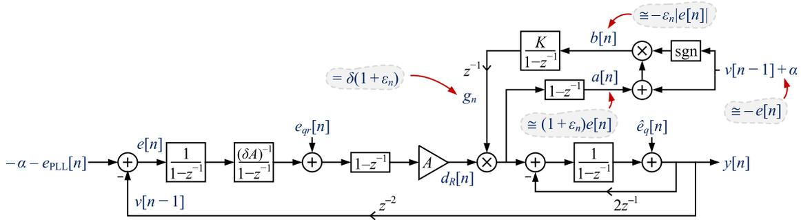
Fig. 7. Rearranged version of the behavioral model shown in Fig. 5(a) modified to accommodate the proposed gain calibration technique.
