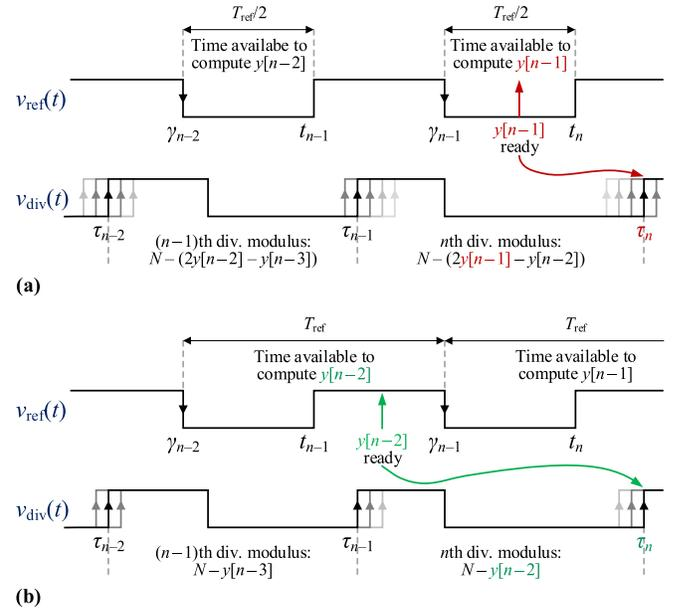
Fig. 4. Example timing diagram of (a) the original  $\Delta\Sigma$  FDC and (b) the proposed  $\Delta\Sigma$  FDC.
