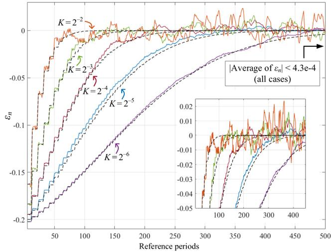
Fig. 10. Sequence  $\epsilon_n$  as a function of  $n$  for several values of  $K$ , where  $\epsilon_n$  calculated via (29) is plotted as a dashed curve for each case.
