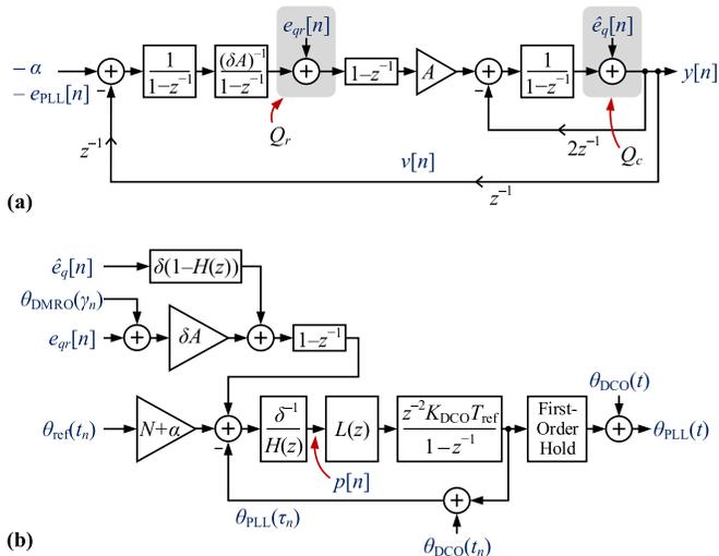
Fig. 5. (a) Behavioral model of the proposed  $\Delta\Sigma$  FDC with (13), where  $Q_r$  and  $Q_c$  are replaced by the additive error sources  $e_{qr}[n]$  and  $e_q[n]$ , respectively, and (b) linearized model of the  $\Delta\Sigma$  FDC-based PLL shown in Fig. 1 with the proposed  $\Delta\Sigma$  FDC and (13).
