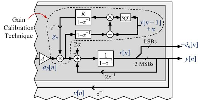
Fig. 6. Digital gain calibration technique shown in the context of the proposed DMRO-based  $\Delta\Sigma$  FDC architecture.
