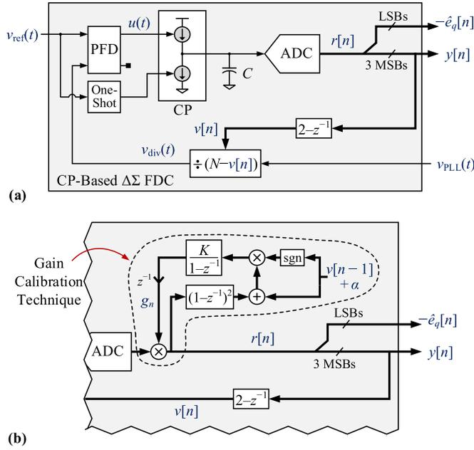
Fig. 8. (a) Simplified block diagram of CP-based  $\Delta\Sigma$  FDC, and (b) digital gain calibration technique shown in the context of the CP-based  $\Delta\Sigma$  FDC architecture.
