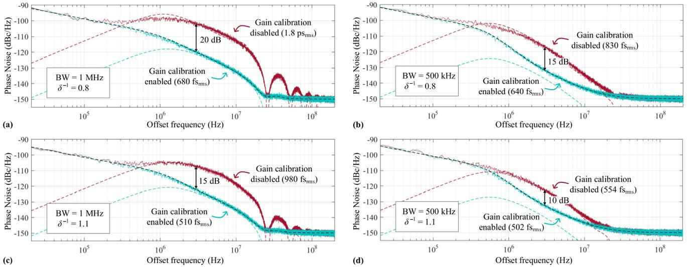
Fig. 9. Simulated PLL phase noise PSD with and without gain calibration enabled for four combinations of PLL bandwidth (BW) and  $\delta^{-1}$ . The black and colored dashed curves correspond to the theoretical phase noise PSD for  $g_n = \delta$  and the combined contribution to the PLL phase noise from  $e_{qr}[n]$  and  $\hat{e}_q[n]$ , respectively.
