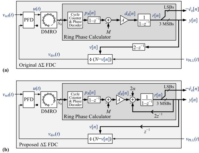
Fig. 2. (a) Simplified block diagram of the DMRO-based  $\Delta\Sigma$  FDC described in [11], and (b) simplified block diagram of the proposed  $\Delta\Sigma$  FDC.
