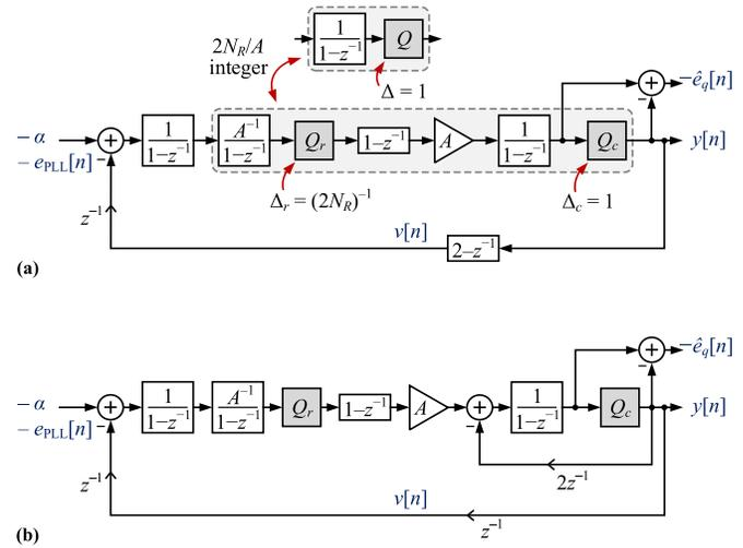
Fig. 3. Signal processing equivalents of the  $\Delta\Sigma$  FDCs shown in Fig. 2(a) and Fig. 2(b) when they are locked.
