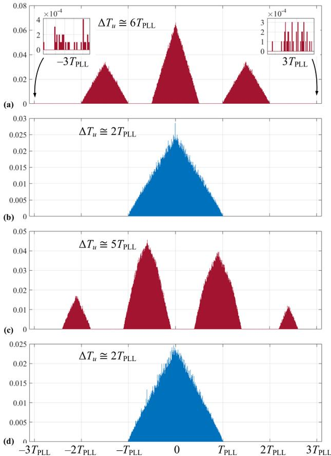
Fig. 11. Normalized histogram of  $u(t)$  pulse width minus  $T_{\bar{u}}$  calculated via (7) for the original FDC [(a) and (c)] and the proposed FDC [(b) and (d)], where  $\alpha = 0.001008987426758$  for (a) and (b) and  $\alpha = 0.401008987426758$  for (c) and (d).
