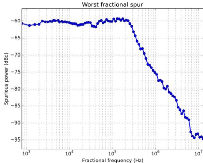
Largest measured fractional spurious tone powers for several fractional frequency settings ranging from 800 Hz to 13 MHz
