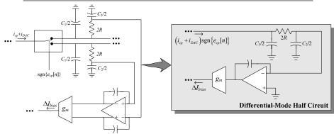
The calibration loop is controlled by a differential-mode signal that has no DC component
