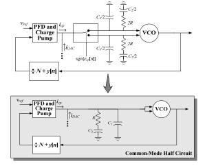
The VCO output is insensitive to calibration signal
