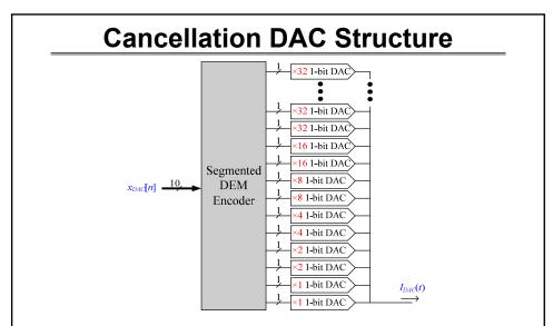
Segmented dynamic element matching used to eliminate harmonic distortion from non-ideal DAC weights and pulse shapes (extension of that in [Chan & Galton, ISSCC 06])
