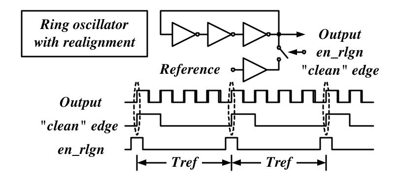
Periodically realigning the oscillator to a "clean" edge suppresses noise accumulation
