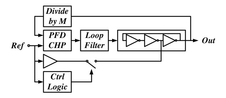
Conventional integer-N PLL except the VCO phase is realigned periodically to a buffered reference edge
