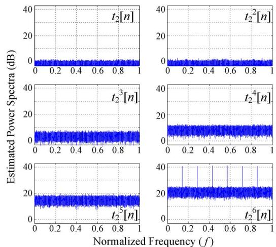
Fig. 5. Estimated power spectra of an optimal quantization noise running sum sequence bounded by 3 when raised to different powers.
