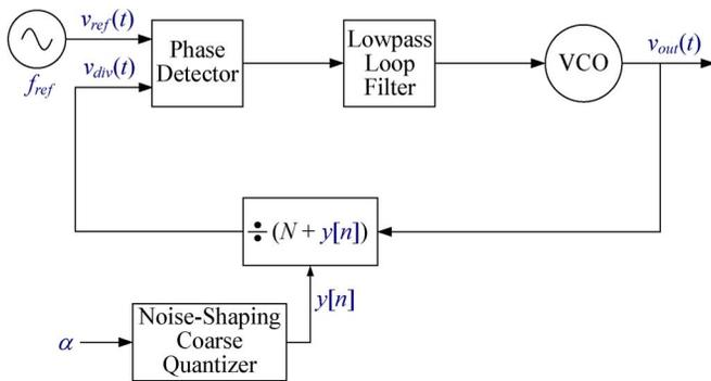
Fig. 1. Block diagram of a fractional- $N$  PLL.
