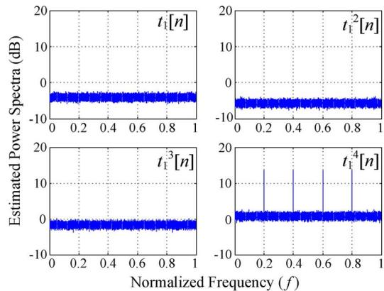
Fig. 4. Estimated power spectra of an optimal quantization noise running sum sequence bounded by 2 when raised to different powers.
