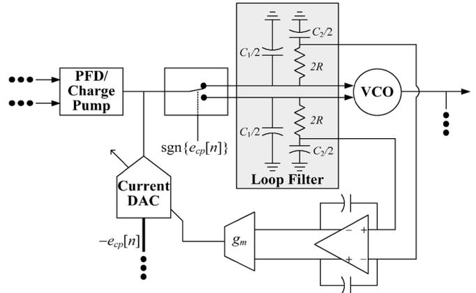
Fig. 5. Block diagram of the proposed adaptive calibration technique.
