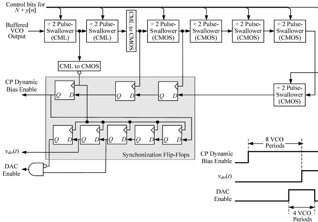
Fig. 8. Divider architecture.
