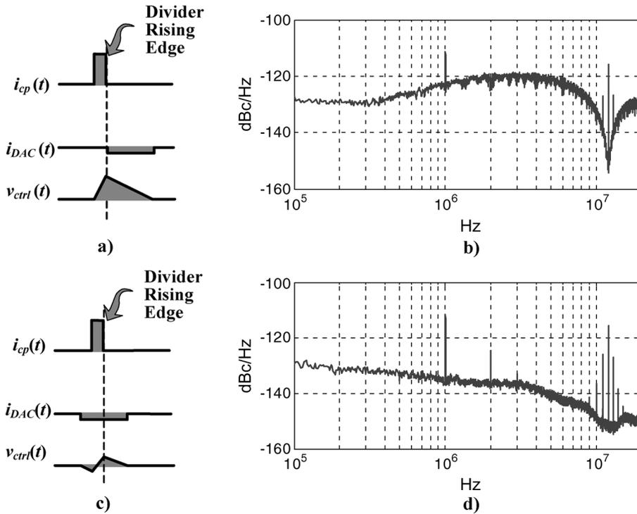
Fig. 9. (a) DAC pulse aligned with divider rising edge. (b) Simulated PLL phase noise for DAC pulse timing in (a). (c) DAC pulse overlapping divider rising edge. (d) Simulated PLL phase noise for DAC pulse timing in (c).
