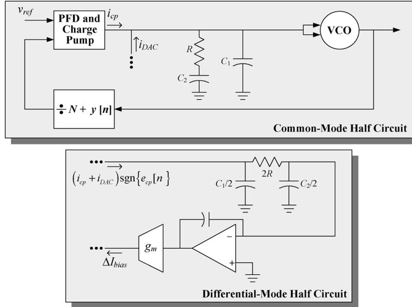
Fig. 6. Half-circuit representations of the PLL and the LMS calibration loop.
