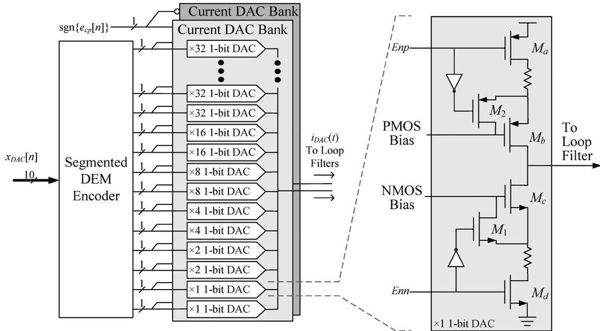
Fig. 10. DAC architecture and circuit.
