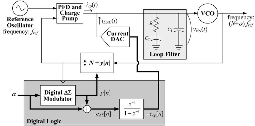
Fig. 2. Block diagram of a phase noise cancelling fractional- $N$  PLL.
