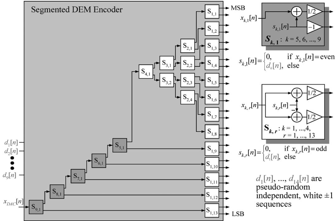
Fig. 11. Segmented dynamic element matching encoder.
