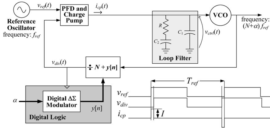
Fig. 1. Block diagram of a fractional- $N$  PLL.
