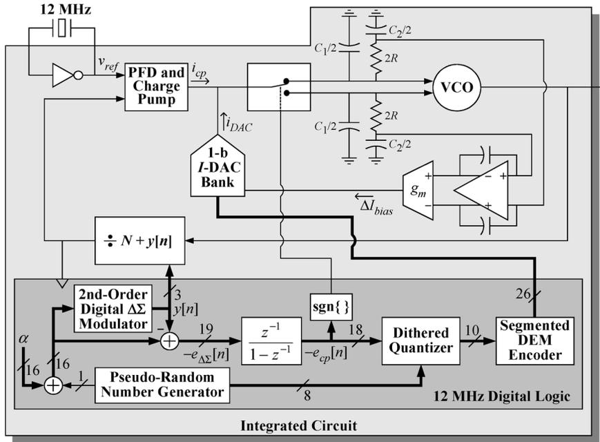
Fig. 7. Block diagram of integrated circuit.
