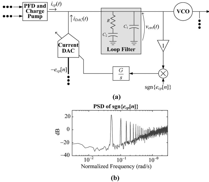
Fig. 4. (a) Block diagram of the adaptive calibration technique proposed in [5]. (b) Simulated discrete-time PSD of the sign of  $e_{cp}[n]$ .
