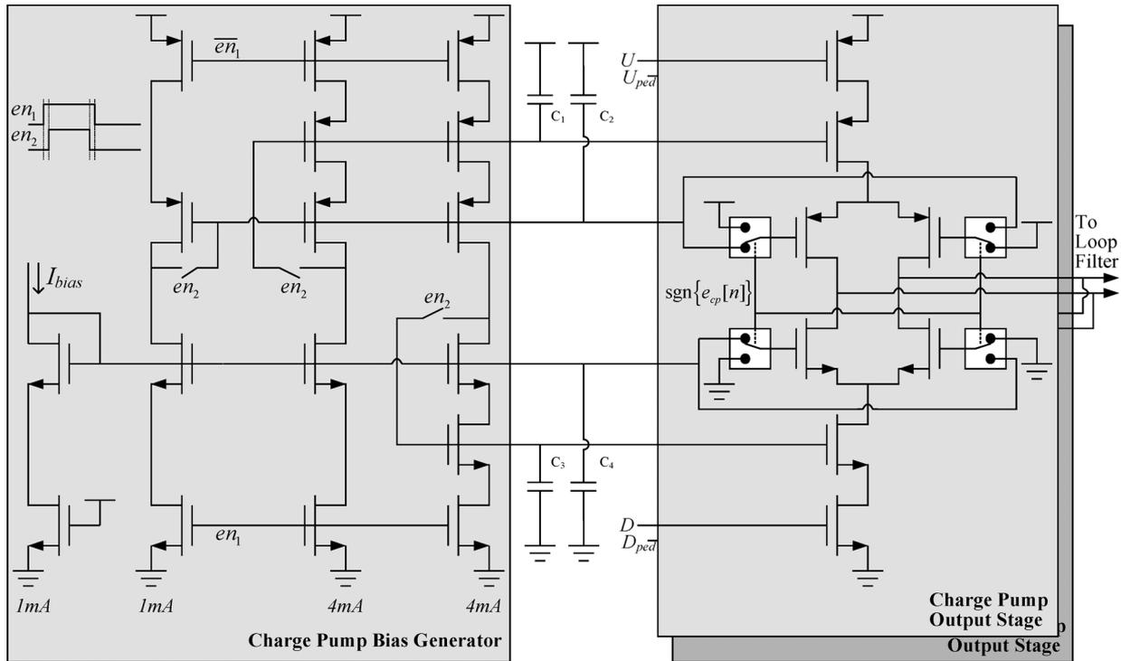
Fig. 12. CP circuit with dynamic bias technique.
