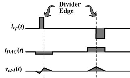
Fig. 3. Effect of cancelling pulse-width modulated charge pump pulses using pulse-amplitude modulated DAC pulses.
