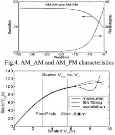
Fig.5. Scaled output magnitude vs. input magnitude
