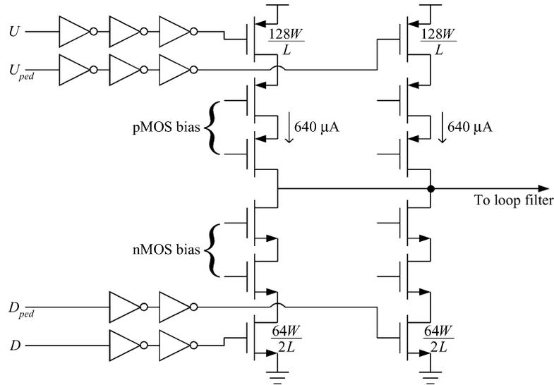
Fig. 11. Modified charge pump circuit.
