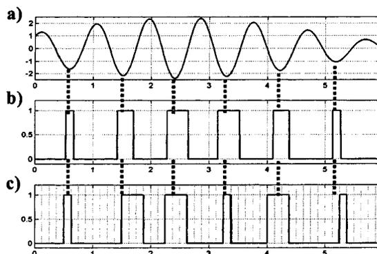
Fig. 1: Representative RF pulse modulated waveforms: (a) Desired microwave signal; (b) RF pulse modulated waveform; (c)  $\Delta$ - $\Sigma$  RF pulse modulated output.
