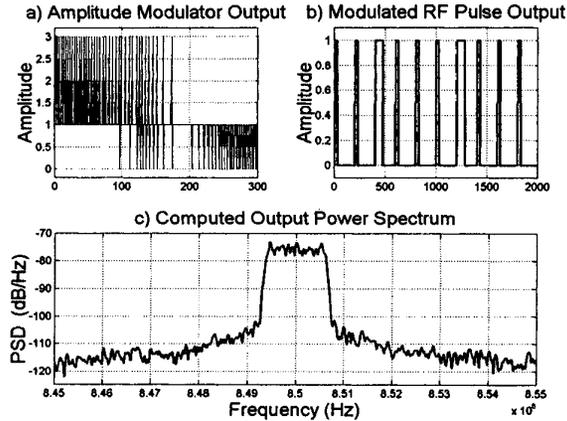
Fig. 4: Simulated waveforms for full CDMA modulation.
