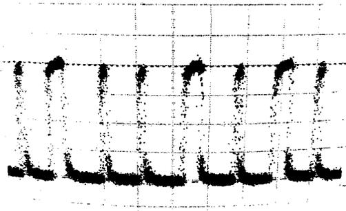
Fig. 5: Measured digital output data stream (scale: 2nS per division, 200 mV per division).
