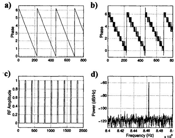
Fig. 3: Simulated waveforms for phase modulator: (a) Input phase vs. time; (b)  $\Delta$ - $\Sigma$  modulator output vs. time; (c) RF pulse position modulated output vs. time; (d) Computed output power spectrum of RF pulse.
