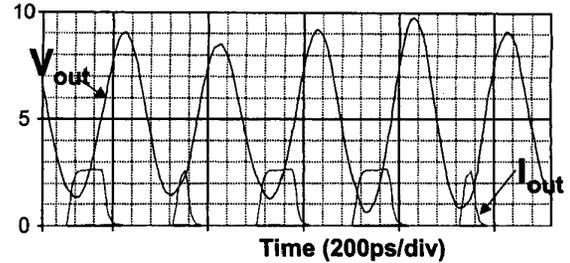
Fig 8: Simulated waveforms for Class C amplifier, driven by RF pulsewidth modulated signals.
